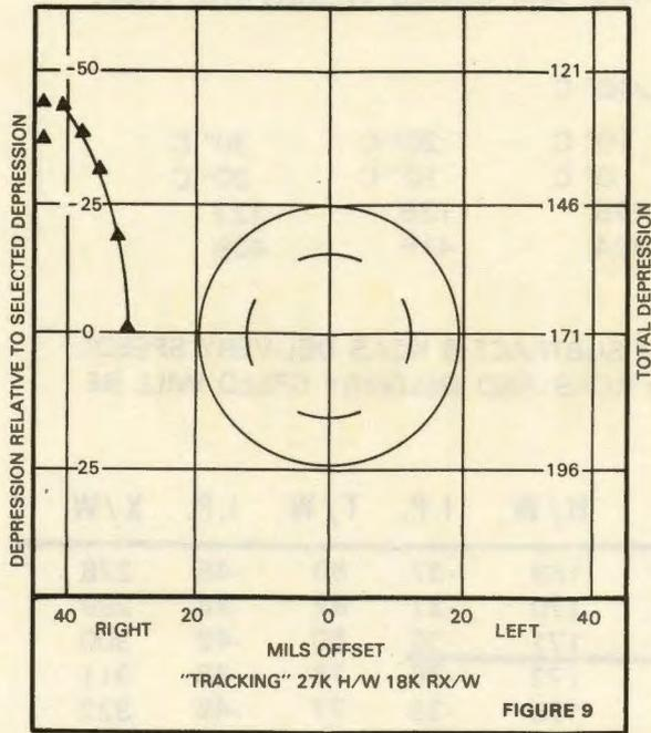
foot circles around them. The final offset is 36 mils and the initial offset is roughly 1.25 times that - or 45 mils. Figure 9 shows the initial pipper placement in relation to the target. "Tracking" until release is also depicted.
